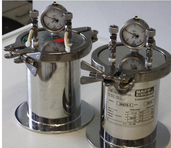
Figure 11. Two customized stainless-steel jars from Raff + Grund (Freiburg am Neckar, Germany) for cultivation of anaerobic autotrophic microbes on solidified medium plates with a pressure capacity of up to 2 bar over-pressure and maximal handling temperature of -10^{\circ}\text{C} to +80^{\circ}\text{C} .
