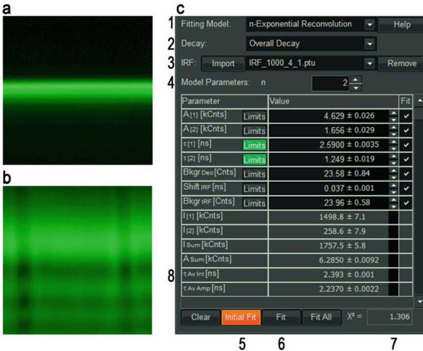
Fig. 5 Comparison between the edge of (a) the upper coverslip which is needed for measuring the IRF and (b) the edge of the microscope slide which should not be measured. (c) Section of SymPhoTime 64 software for evaluation of FRET-FLIM data. (1) The “Fitting Model” should be “n-Exponential Reconvolution” while the (2) “Decay” should be “Overall Decay.” (3) The experimentally measured IRF (Subheading 3.8.6) has to be imported here (4). “Model Parameters – n” have to be set up according to the decay variant of the donor. Calculation is started with (5) “Initial Fit” and (6) Fit (7). If \chi^2 is in the range of approximately 1–2, the fluorescence lifetime \tau in [8] can be copied for further evaluation
