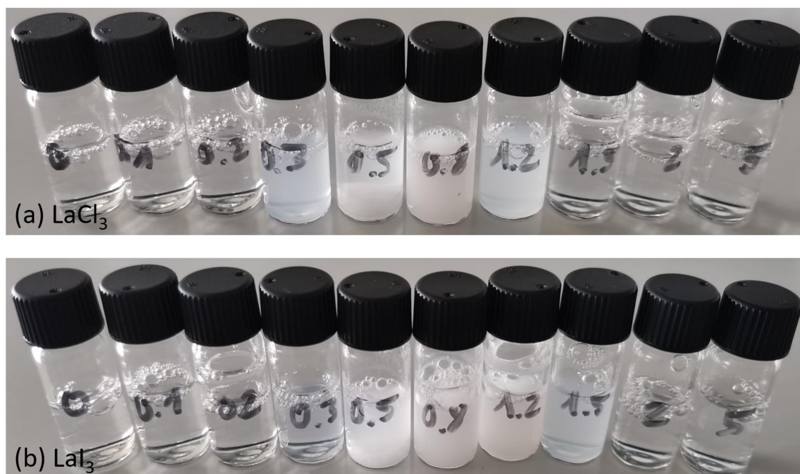
Figure 8.2: Phase transitions. Dilution series at 5 mg/ml BLG and room temperature with (a) LaCl 3 and (b) LaI 3 in H 2 O. The bottles are labelled with the respective c_s in mM.
