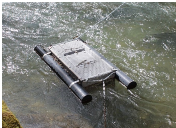
Figure 1: Cage used for in situ exposure of rainbow trout.
