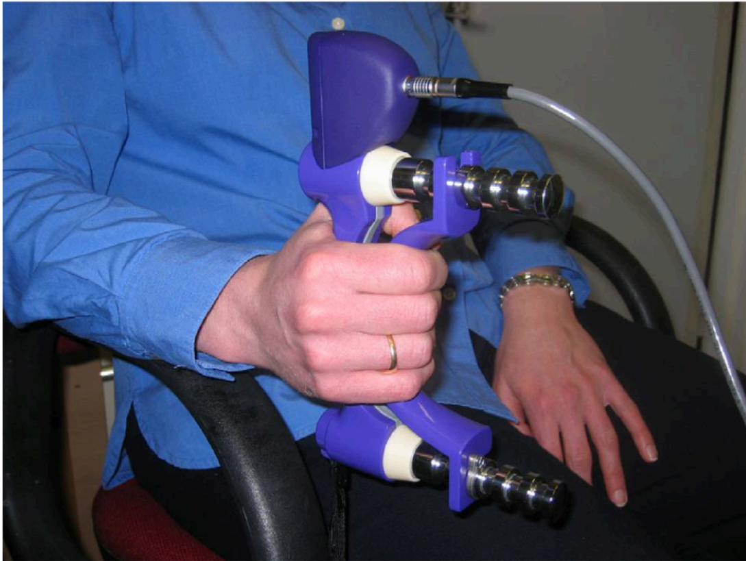
Abb.13 Dynamometer [55] (Biometrics Ltd, Newport, England)
