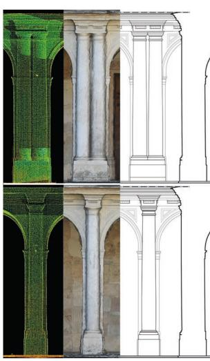
**Figure 5.** Construction of real 3D/2D models of the half column and the binate column.
