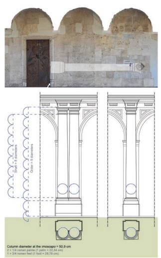
**Figure 8.** Proportion of the architectural order. The half column and the binate column. The total length of the order matches the distance between tracing 2 and the jamb of the left door of the church.
