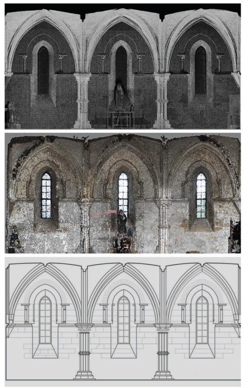
**Figure 6.** Architectural scale, the Chapter House: numerical model derived from laser scanning, numerical model derived from Structure from Motion and Image Matching, architectural 2D model.
