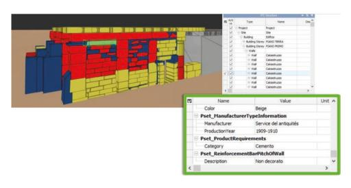
Figure 5. Building Information Modeling is used in order to associate additional information, such as alphanumeric data (e.g. date, material, state of degradation, management of restoration, etc.) or other files (e.g. images, archival documents, etc.) to building components. In this case, the BIM model of the Temple of Amada (Archicad 20 and IFC Viewer BIM Vision software).
