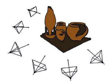
**Figure 1.** Image acquisition planning: ideally the pictures need to be taken moving around the vertical axis of the object at  $360^{\circ}$  for isolated objects and  $180^{\circ}$  for flat ones, with the camera oriented in the range of  $30^{\circ} / 45^{\circ}$ .
