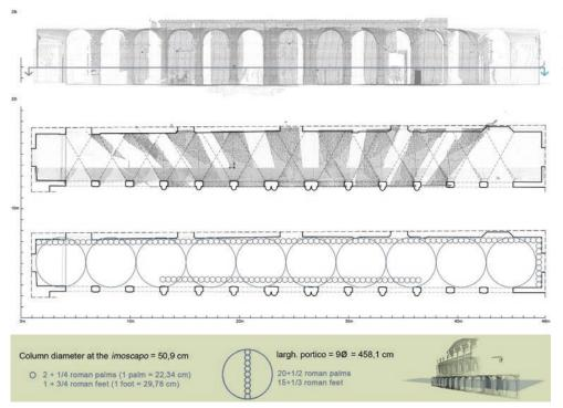
**Figure 10.** Proportion of the portico. The length, 46.31 m, corresponds to 91 modules; the width, which varies between 4.27 m on the left and 4.61 m on the right, completely match 9 modules in the central part of the facade, axis with the main portal.
