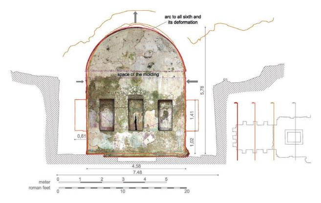
Figure 9. Transversal section in which some particular features of the *nymphaeum* are highlighted.
