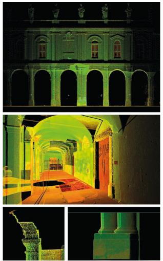
**Figure 3.** Surveying of the architectural complex. The structured point cloud of the church obtained by laser scanner surveying.
