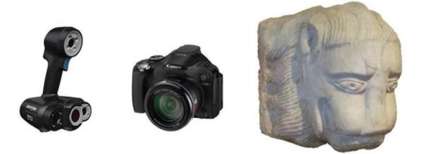
**Figure 4.** Structured light 3D scanner Creaform GO!Scan50 (left) and DSLR camera Canon PowerShot SX30 IS (centre). Test case: italic marble lion's head, "Doccione di fontana" (right), Galleria Nazionale dell'Umbria di Perugia, Italy.
