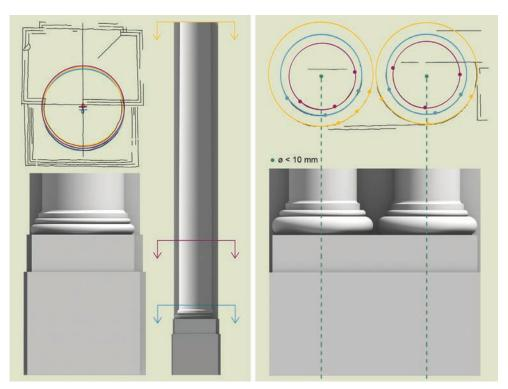
**Figure 7.** Analysis and geometric constructions of the half column and the binate column. For half column, the mouldings have been modeled on the basis of the surveying of the real element and of the tracing 5, since it is not possible to obtain enough information just from the worksite tracing 3.
