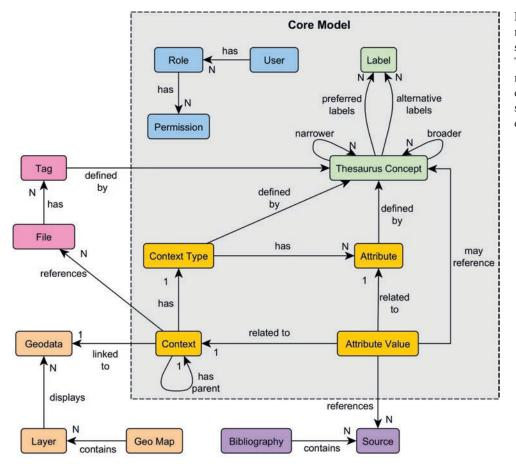
**Figure 3.** Spacialist data model illustrated as a simplified concept model. The core part is contained in the gray box. The extension parts are outside of the gray box and explained in Section 4.3.
