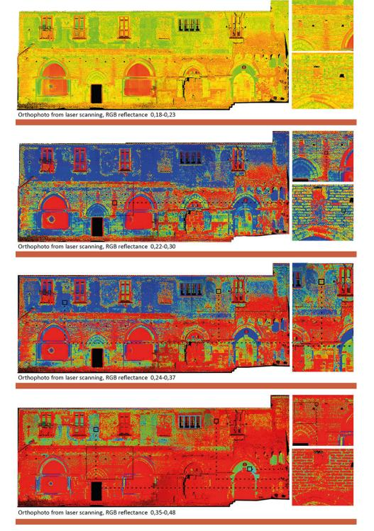
**Figure 10.** Orthophoto of the Façade obtained through laser scanningreflectance mode, into 4 different extensions of the chromatic scale of values.
