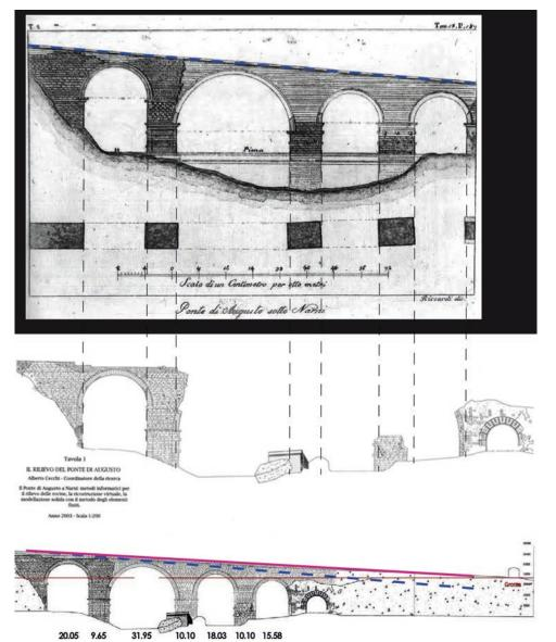
Figure 4. Survey and hypotheses for the reconstruction of the bridge by Eng. Giuseppe Riccardi in 1837. The differences in the springing line of the great arch, the declivity of the street and misalignment of the pillars are clearly visible (from Tattoli 2000). A comparison with Cecchi's survey. The dashed line represent the excessive slope of the road to Riccardi, compared with the slope.
