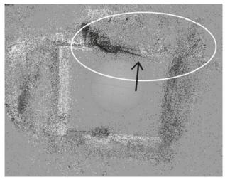
**Figure 4a.** Sparse point cloud of Building 12 from Aigition showing poor alignment at left caused by small baseline distances.
