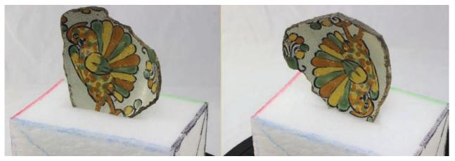
**Figure 5.** Each object was photographed in chunks. The patterned foam block aided the software's in detecting overlap between rotations within a chunk and thereby aligning photographs in three dimensions. This shows the two chunks used to build a model of the Abó Polychrome Majolica Plate.
