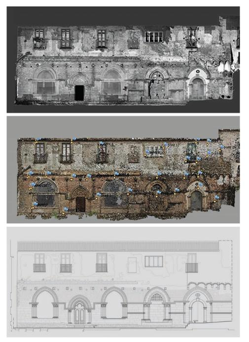
**Figure 4.** Urban scale, the Façade: numerical model derived from laser scanning, numerical model derived from Structure from Motion and Image Matching, architectural 2D model.
