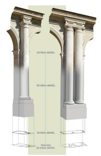
**Figure 6.** Construction of ideal 3D/2D models of the half column and the binate column. The information that could not be deduced from the worksite tracings are integrated with the images of the real elements.
