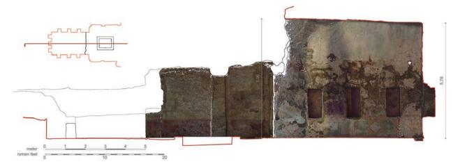
Figure 7. Longitudinal section with the front textured using the spherical panoramas.
