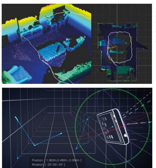
**Figure 3.** Google Tango tracks space in realtime and creates a point cloud. The numerical model is stored on the device memory, and it will update as the real environment changes.
