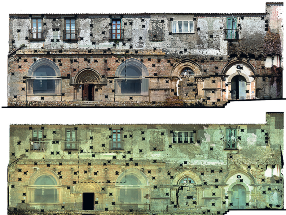
Recognition of homologous point in comparison of the point cloud of 3d laser scanning
