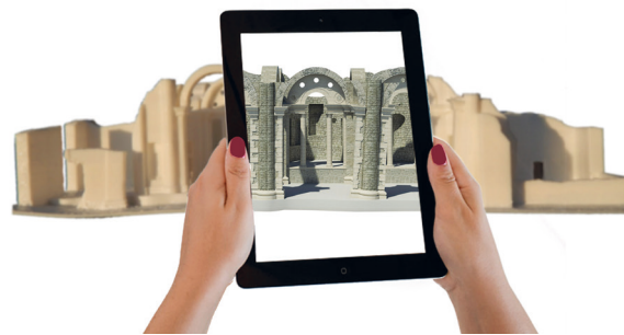
Figure 1. 3D printing and virtual model are overlaid by using mixed reality.
